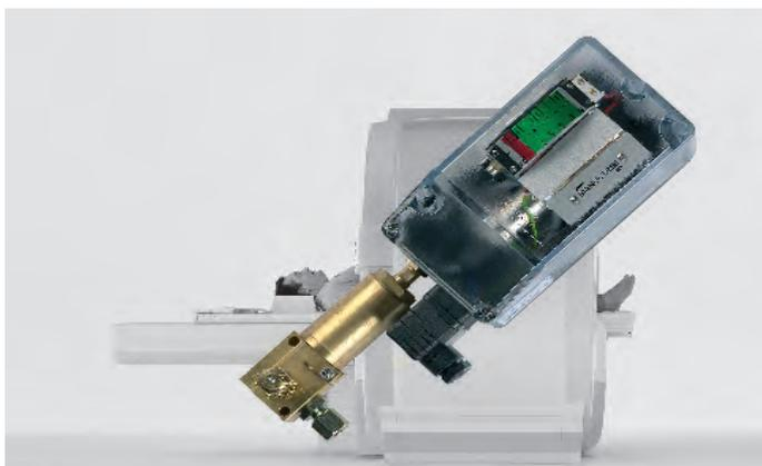
**Special Design Pressure Switch (TÜV)** | This specially designed unit used on MRTs is able to switch 13 mbar on failing helium supply plus it withstands overpressure shocks up to 4 bar without any malfunctions. The integr. pressure transducer is used for signalling to a PLC and the integr. pressure gauge tells the service personell if the system is pressurized even when there is no power supply.
