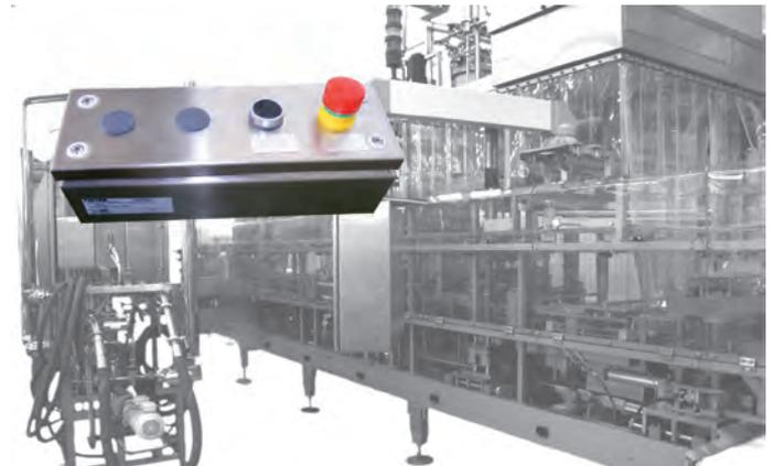
**Emergency Stop Module for General Engineering (ATEX, PL) |** The ESM was developed and is being manufactured for a customer making high-pressure compressors. It provides an out-the-box solution for stopping the compressor from working in an emergency situation. Kept simple, the machine operator just has to hit one STOP-button for a controlled shutdown.
