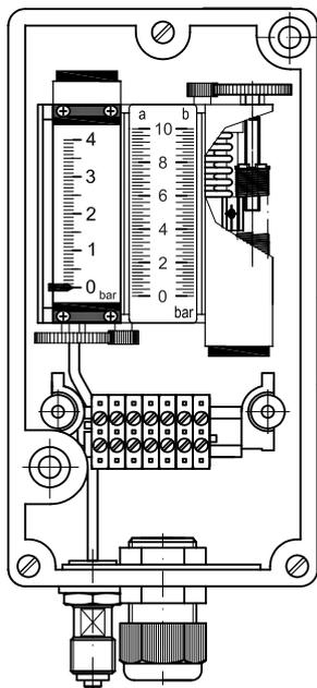
Mechanical force-balance measuring system with bellows sensor actuating one or two switching contacts, featuring:
