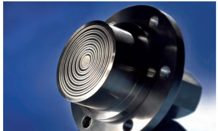
**Diaphragm Seals** | Mechanical process separating elements which are mounted on measuring instruments directly or via capillary; with diaphragm seals the measuring instrument is separated from the actual process to protect the instrument from hot, polluted, aggressive or chrysalizing media.
